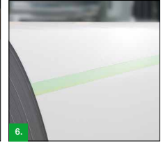
Figure 5 + 6: Remove the lower part of the liner from the tape before accelerating the reel.
