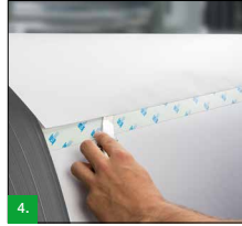
Figure 4: Fold back and remove excess paper tail.
